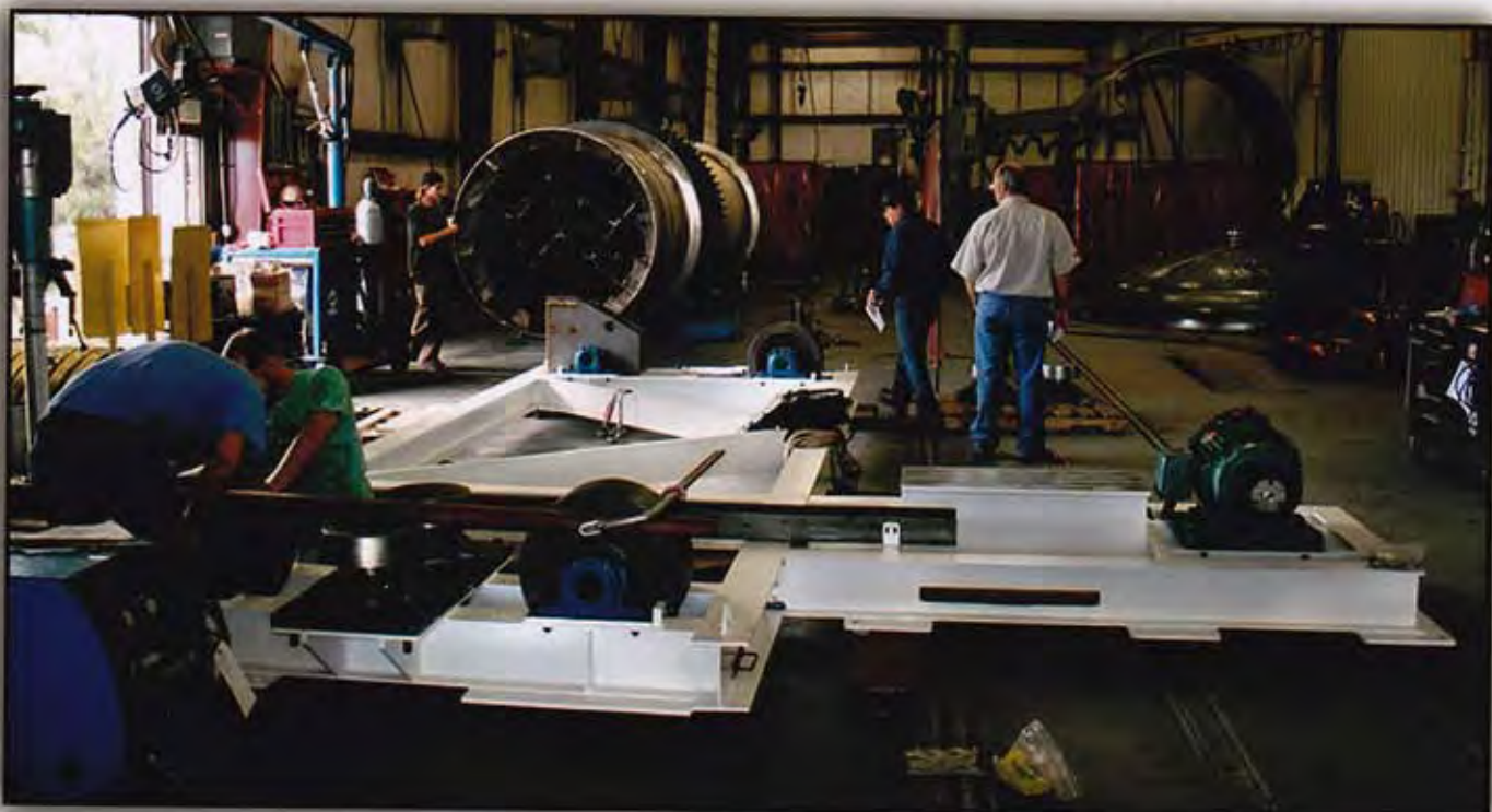
First Drum - tires in location, sprocket being match drilled
