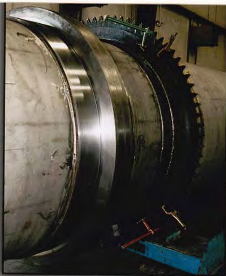
First Drum - tires in location, sprocket being match drilled
